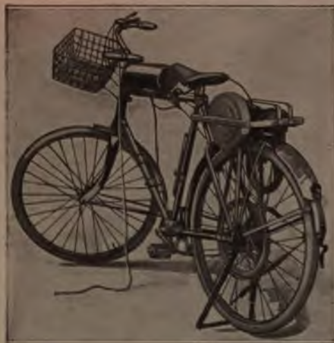
An Itinerant Cutlery Grinder has Adapted a Motor-Driven Bicycle to Meet the Requirements of His Calling by Attaching a Grinding Wheel
